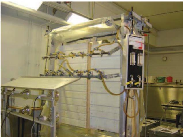
The boards fitted from both edges using fastenings which were 75 mm length nails so that the pith side of the board located in the front side. The test period consisted of 7 wetting and drying periods. In a wetting period, the surface of the element was wetted using a driving rain test apparatus, which sprayed 1.35 l/m<sup>2</sup>/h to the surface for 3 hours. After wetting period, the element was exposed to drying at 30±5% RH for 21 hours.
